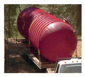
that could be used for parking or other needs, and it makes the property aesthetically pleasing. Also, since the tank is buried, it does not require the expensive protection against water freezing that might be necessary with an aboveground tank.
